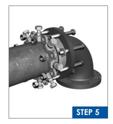
Assemble the joint using supplied flange bolts. Torque all flange bolts in alternating manner as per the torque values given in the table. Make joint deflection if required before actuating torque off bolts. Joint deflection must not exceed the given values and must not make the separation any more than max. allowable distance "D."
