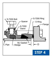
Move the pipe towards the flange face bringing it within max. allowable distance "D" from flange face. Refer to Table A for max. allowable distance "D" and Max. allowable deflection of pipe.
