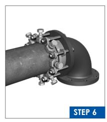
Tighten torque off bolts in an alternate manner such that all wedges touch the pipe. Never turn a single bolt over 180 degrees without alternating to another bolt.
