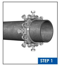
Pipe to be cut to required length and surface to be clean. Insert 7200 gland assembly with lip of the gland facing the plain end of pipe.
